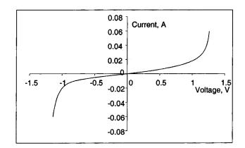
FIG. 3. Typical I-V curve for an Al/a-CdTe:O/Pb tunnel junction. The slope change from 0 V to approximately  $\pm 0.6$  V is typically 10%–30% and is asymmetric with bias polarity.
